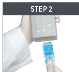
Close and insert the cartridge into the i-STAT .
